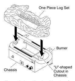
Figure 25 - Installing One-Piece Log Set
